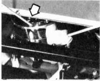
drum (see arrow). Got that? Okay. Now you can take a clean swab and perform the same operation on the stationary heads used for audio, erase, and control track. And don't forget the tape guides, which often wind up with some oxide residue.
