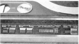
All of the Magnavision's controls are neatly a rayed in one continuous horizontal row. Pictured above are the still-frame stepping, slow motion, and standard play controls.
