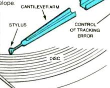
In the electro-tracking system, coils at the base of the cantilever arm receive error correction signals. The arrangement permits the arm to move transversely and longitudinally, thereby correcting for tracking and time-base errors. User commands and special effects are also mediated via this system.
