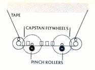
Pioneer's Closed Loop Daar Capsian Tape Transport System ensures constant tape to he id contact
