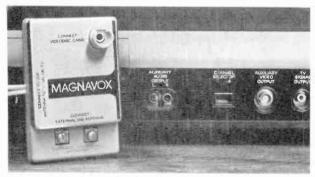
A separate signal-splitting box (lef.) is necessary to accommodate the Magnavision's output as well as normal antenna or cable-TV feeds. High-quality stereo signals are available via left and right channel audio output jacks.
