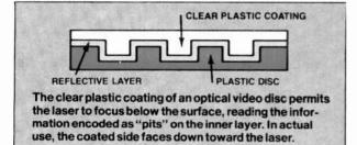
plastic coating are invisible to the pickup circuitry. That's true to a degree, but precautions still must be taken. Like audio records, video discs are susceptible to warp and should be stored away from sources of heat. Though fingerprints and dust are largely ignored by the player, cigarette ash, bubblegum, and the like are not.
