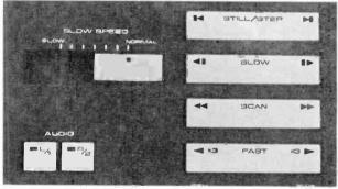
Controls on the Laser Disc player are grouped on the top plate. Pictured above are still-frame stepping, slow motion, fast scan, and triple-speed cor trols.
