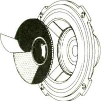
And since the glass fiber is non-porous, it gives our air suspension speakers a perfect seal, and a lower resonance frequency for better bass response.
