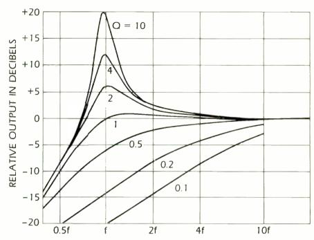
Response curves for differing values of Q show that at a Q of 0.75 to 1 a speaker's output at resonance frequency (f) is flat in relation to output above.
