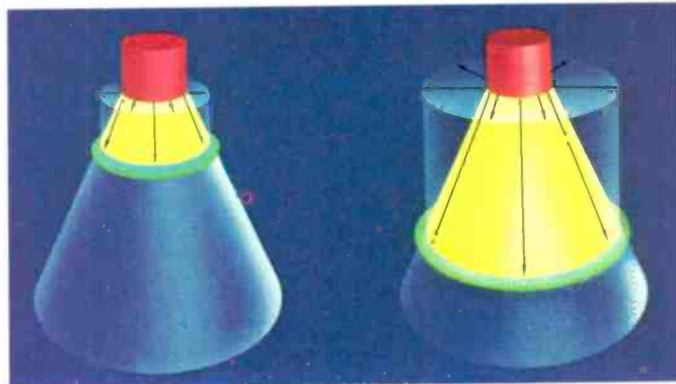
Since all frequencies radiate in a 360° pattern from a single driver in the Ohm F, there is perfect horizontal dispersion with no time delay distortion.
