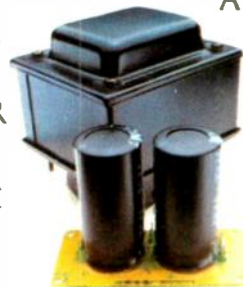
DC power supply found on the most expensive receivers.
