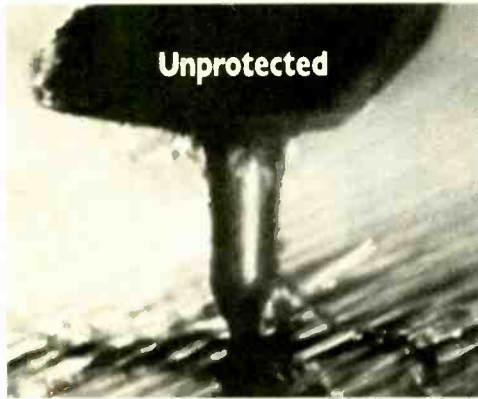
Magnification shows the record vinyl wearing away.
