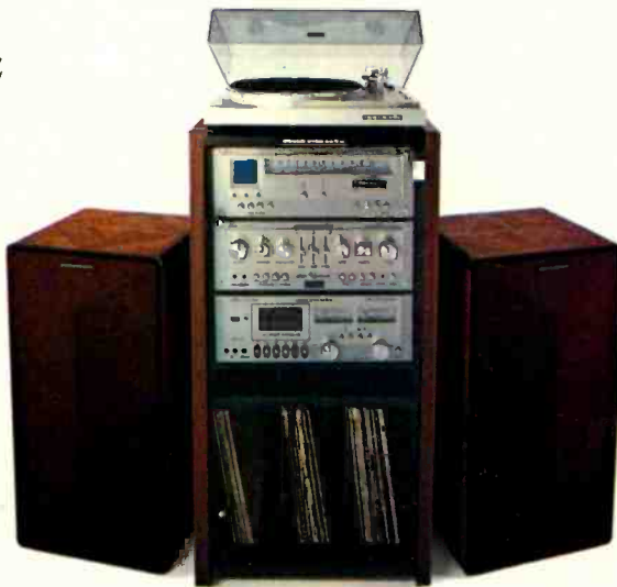
The RM-3700 STACK RACK contains three Marantz components on fixed-positioned shelves, an accessory shelf and divided record compartment behind its full-length smoked-glass door. The Marantz system shown includes the 6170Q Turntable, 2110 Tuner, 1180DC Integrated Amplifier, 5010B Cassette Deck and Design Series 930 Speakers.
