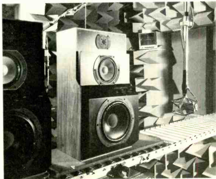
Anechoic chamber in B&W production line, Worthing, Sussex
