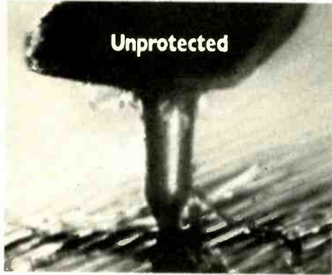
Magnification shows the record vinyl wearing away.
