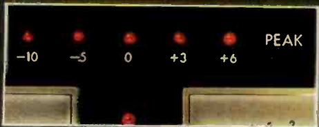
5 LED peak level indicators help eliminate distortion.
