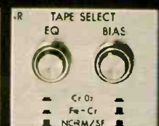
Bias and EQ switches for all types of tape.
