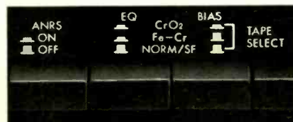
Automatic Noise Reduction System reduces tape hiss.
