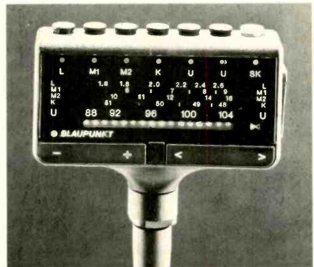
Blaupunkt's $1,200 Berlin system includes a control box (shown here), a cassette deck, and a separate receiving unit.
