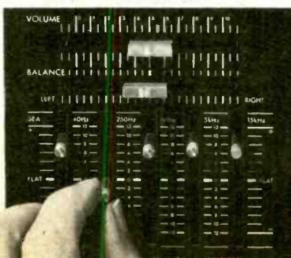
5-zone SEA graphic equalizer system offers tone adjustment over entire musical range.
