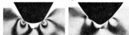
Stress analysis photos show concentrated high pressure with elliptical stylus (left), reduced pressure, less groove distortion with Shibata stylus (right).
