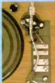
S-shaped tonearm for ideal tracking
