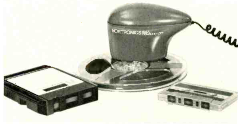
Recordists welcome degaussing gear—either bulk eraser like Nortronic's (left) or head degausser like Nakamichi's (below).
