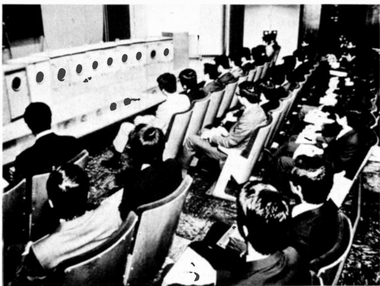
Toshiba is among the companies using closely controlled group experiments to determine speaker-design criteria.
