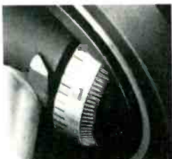
Stylus pressure dial calibrated in tenths of a gram from 0 to 1.5 grams; in quarters of a gram from 1.5 to 3.0 grams.
