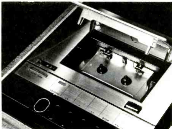
Cassette-well cover opens wide for cleaning and degaussing. Base plate at bottom of well pops up to eject cassette, can be pressed down (as it is here) for servicing. Note "tape run" light at far left.
