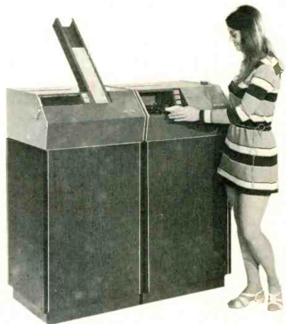
Present (perhaps temporary?) state of the art: Ampex says this $10,000 stereo cassette duplication system, which drives both master and copies at 75 inches per second, is "five times faster than any previous cassette duplicator."
