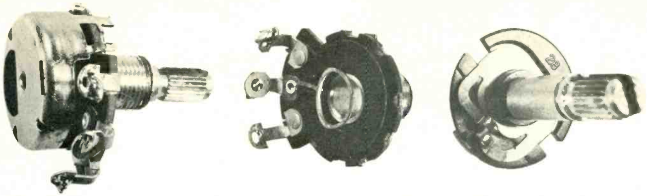
Fig. 2. The anatomy of a potentiometer (familiarily, a "pot"). At left, the complete device with its three connecting lugs and rotating shaft. The two end lugs get the full voltage since they are connected directly to the internal resistive element (see center photo). At right, the rotating member with its metallic wipers. One wiper contacts the resistive element at a particular point, depending on how the shaft is rotated. In this way the center lug becomes connected to the resistive element, and the point of connection—and hence the amount of resistance in the circuit—can be continuously varied at will.
