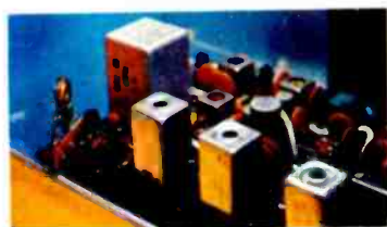
4 ICs and Crystal Filter FM IF Stages deliver superb selectivity and 1.5 dB capture ratio
