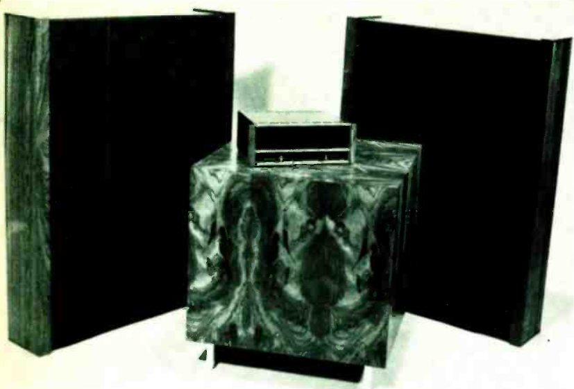
Servo-Statik I system consists of two electrostatic panels for left and right channel frequencies above 110 Hz, a mixed-channel bass reproducer housed in commode, and an electronic unit that contains the servo/bass amplifier, electronic crossover, and level controls for highs and lows.
