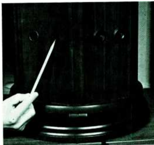
Wooden plugs may be removed from rear panels to augment bass response of Empire speaker system.
