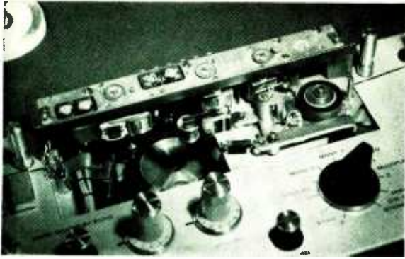
With head covers removed, bias and playback level adjustments on Uher 10,000 are visible as pairs of screw-driver controls on head mount. Heads are for erase (at left), Dia-Pilot, record, playback.
