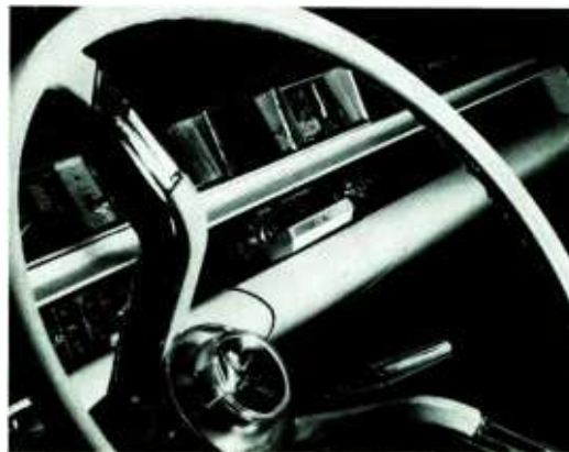
Lear system employs unique eight-track cartridge; is part of radio offered by same manufacturer.
