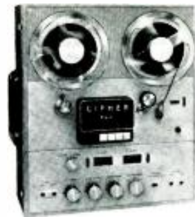
CIPHER 800 a professional 4-track stereo recorder with 3 hysteresis-synchronous motors and 3 heads; plug-in head assembly (2-track also available), no pressure pads, tape speeds 7\frac{1}{2} and 3\frac{1}{2} ips, solenoid controlled, 2 VU meters, $499.95.
