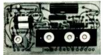
Driver stage: Wideband silicon driver transistors are mounted on rugged, military-type epoxy glass board. Board pivots for easy accessibility or removal.
