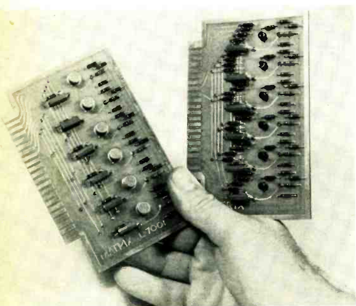
Transistors suggest an increased use of printed circuit subassemblies, which are compact and neatly laid out.
