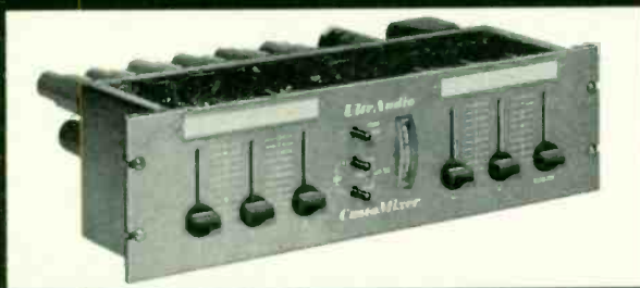
Model M-5: Five independent mixing positions plus master gain control. Phono equalizing and cueing switches on front panel for mixers 2 & 3. A 60db pad switch enables mixer-1 to accept a high level, low impedance source. Single channel output.
