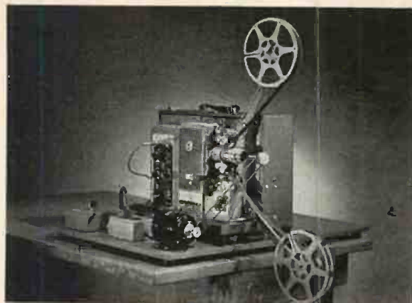
Figure 3. This is Kodak's MK4 Pageant projector, shown with synchronous motor which guarantees constant speed.
