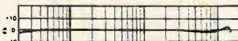
Model RG-555 Cartridge Frequency response 33 1/2 rpm record with compensation for Decca curve.
