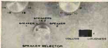
Three position speaker-selector switch lets you use either of two speaker systems, or both at once.
