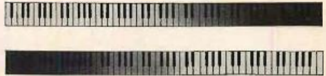
Fig. 3a. A low-pass filter suppresses treble and passes bass tones. Fig. 3b. A high-pass filter passes treble but removes bass tones. A combination of these will give selective coverage of the full audible range.
