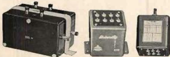
Fig. 1. Three typical speaker system dividing networks. On the left is a Stephens 800-cycle network; the others are universal networks made by University Loudspeakers.
