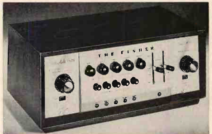
The 90-C is equipped with mixing controls.
