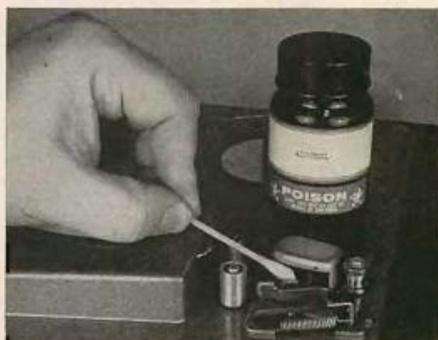
Heads, head guides, and pressure pads should be cleaned often with alcohol or special fluid. Follow instruction book.
