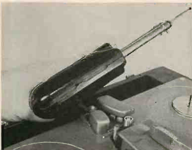
A head demagnetizer should be used often. If you don't have one, your soldering iron will serve as a temporary substitute.
