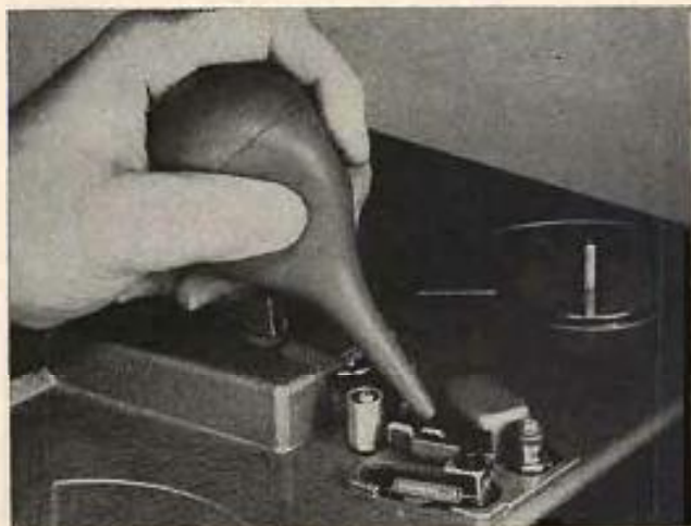
Between periodic liquid-cleaning operations keep machine free of grit by blowing it away with syringe or similar tool.
