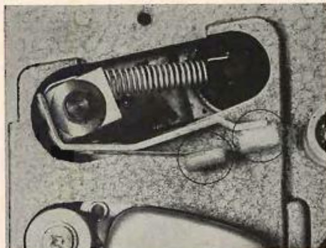
If your machine has pressure pads such as these, keep them soft by regular cleaning: replace them when wear is severe.
