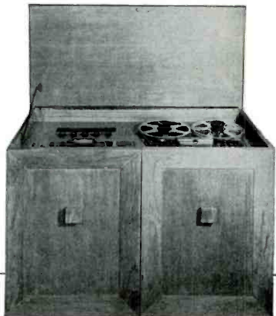
An Ampex in a typical custom-built cabinet containing FM and AM radio, recorder, and disc record changer.
