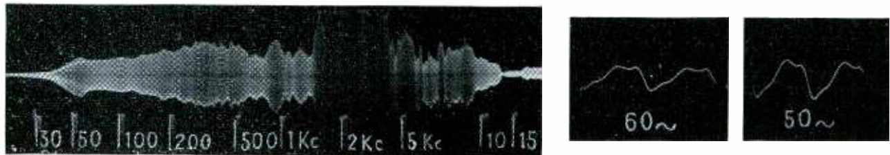
Fig. 6. Free field response curve waveforms of typical 12-in. speaker. No negative feedback; impedance source 100 ohms. Note the bump in the 60-cycle zone and evidence of frequency doubling.
