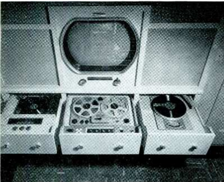
Fig. 2. Three drawers, underneath the television screen, house record changer, FM-AM tuner, tape recorder, antenna and amplifier controls, and transcription turntable.
