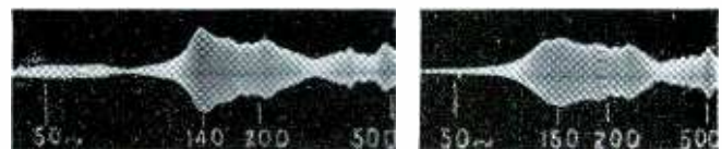
Fig. 14. Intermodulation distortion is shown in the left-hand trace by difference between contours of bottom and top lines. Speaker was 8-in.; input 60 cycles, 2.8 volts. A 1,900-cycle tone was fed in with 60-cycle tone. At right, the 1,900-cycle tone was switched to another speaker; contours of top and bottom lines become the same.
