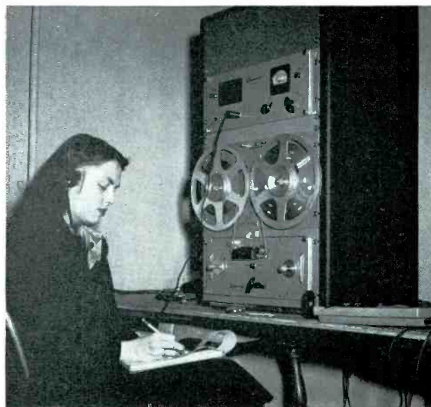
Outside programs can be brought in by telephone line and recorded on this Magnacord machine, monitored by Nancy Maguire.
