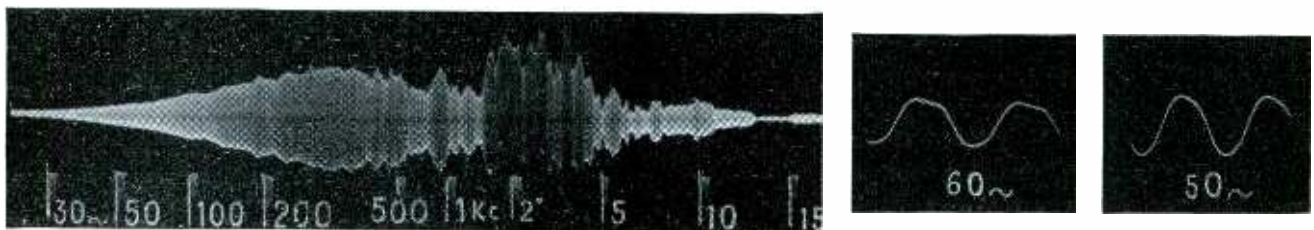
Fig. 7. Conditions same as in Fig. 6 except that 14 db of feedback employed. Cone resonance around 60 cycles has disappeared.
