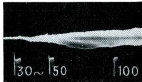
Fig. 3. Oscillogram of free field response of typical 10-in. speaker. Note the difference in the contour of the trace above and below the dark center line. This indicates faulty cone suspension. Input level 1 watt at 500 cycles. Microphone 12 ins. on axis.
