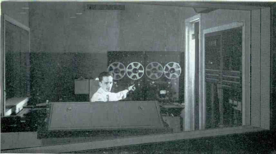
Looking into the control room from the larger studio at Symphony Hall. A Browning FM tuner and an H. H. Scott amplifier are mounted at the top of the racks on the right. These are used for monitoring purposes. Behind the operator are two Ampex machines which provide 15,000-cycle program quality from tape. Above the two transcription turntables on the left is the window which opens into a smaller studio, used principally for interviews.
