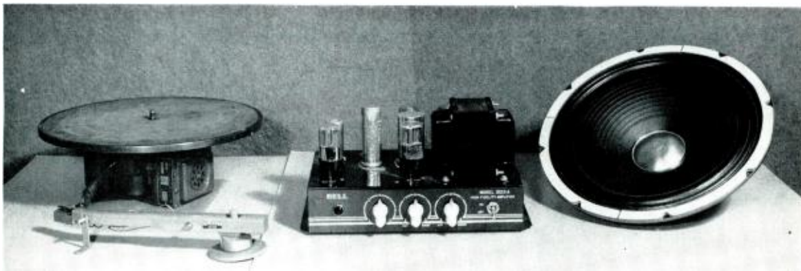
There are only four units in a phonograph system: pickup, turntable, amplifier and speaker.
