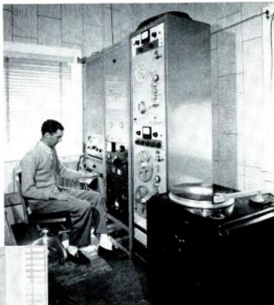
Above: Engineer-operator Ralph Thompson prepares to switch over from a program coming up from Charlotte via the studio-transmitter link to one previously recorded on the tape equipment. The receiver mounted on the left hand rack is used to pick up FM programs from other stations, to be rebroadcast on WMIT.
