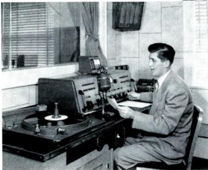
Above: Engineer-operator Ralph Thompson prepares to switch over from a program coming up from Charlotte via the studio-transmitter link to one previously recorded on the tape equipment. The receiver mounted on the left hand rack is used to pick up FM programs from other stations, to be rebroadcast on WMIT.
