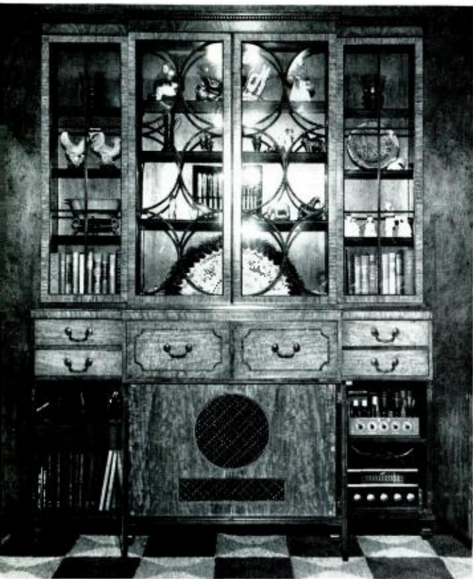
As on page 23, an existing piece of furniture has been used to house the speaker. In this case, all the equipment has been built into this one unit. Equipment includes a Garrard record changer, Altec amplifier and coaxial speaker, Radio Craftsman FM-AM tuner. Installation by Bluff City, Memphis, Tenn.
