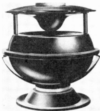
Omnidirectional speaker for reproduction
