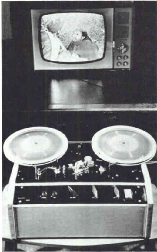
Wesgrove's VKR-500 (below) is a "brute-force" system supplying up to 30 minutes of recording time.
