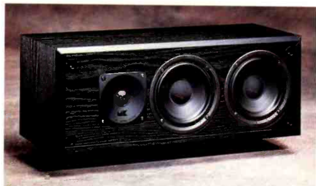
M&K's least expensive center speaker, the Center-75 ($295), features a Phase-Focused crossover and an unusual asymmetrical configuration for its 1-inch tweeter and 5¼-inch woofers; these are said to optimize off-axis response and improve horizontal dispersion. The 18¼ x 7 x 7½-inch (W x H x D) cabinet is finished in woodgrain vinyl. Sensitivity is rated as 90 dB.
