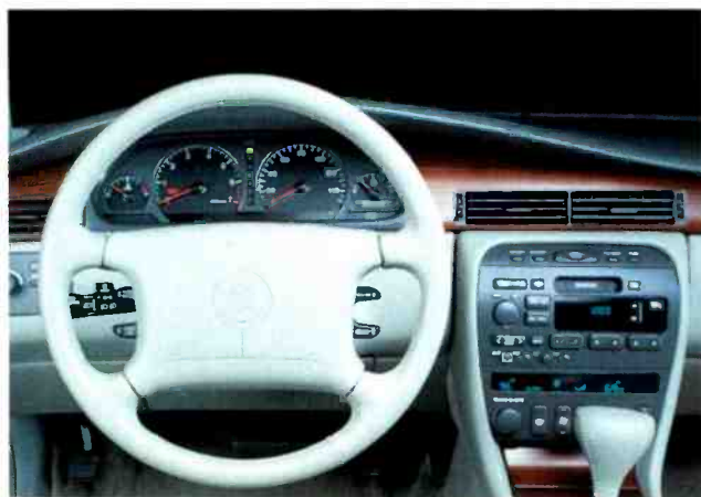
Audio controls are mounted in the steering wheel of the Cadillac Seville Touring Sedan, which is available with an optional Delco/Bose system featuring DSP.
