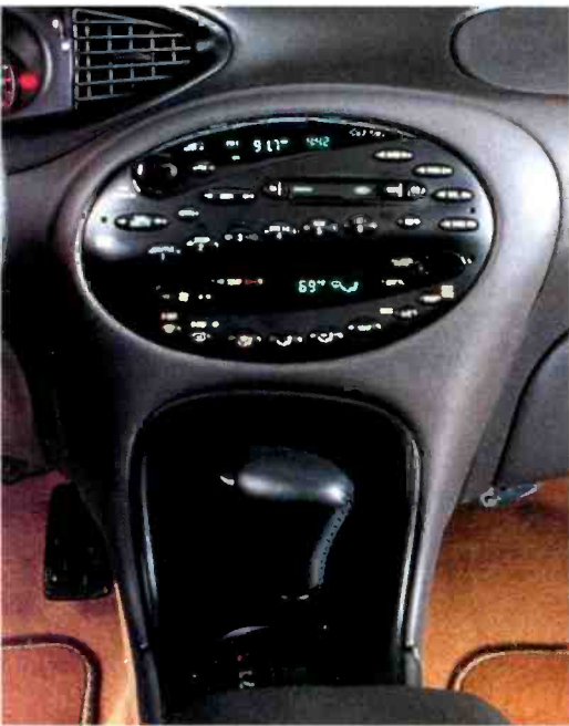
An oval-shaped panel in the Ford Taurus integrates temperature and audio controls, the latter linked to a tuner/amplifier mounted in the trunk.
