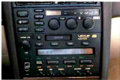
Factory-installed options in the Lexus LS400 include a six-CD changer (mounted behind a door above the glovebox) and a Nakamichi head unit with custom EQ.
