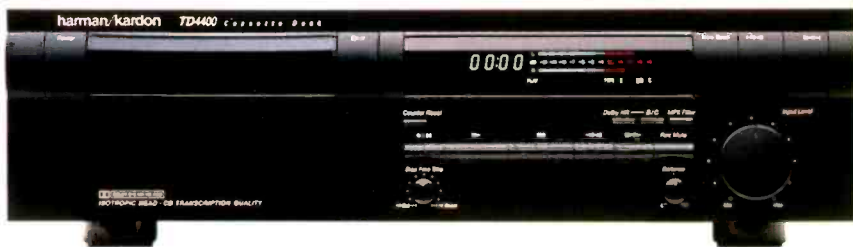
Harman Kardon's TD-4400 ($449) is a two-head deck featuring separate motors for the tape reels and capstan, Dolby HX Pro, Dolby B and C noise reduction, peak-level meters, a bias fine-tune control, a linear time counter, programmable music search, and an intro-scan mode that plays 15-second samples of every song on a cassette.
