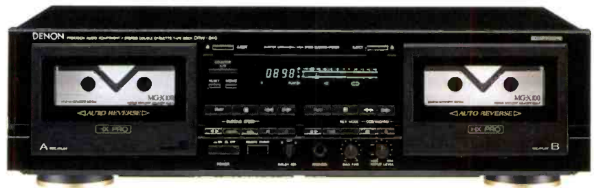
Denon's DRW-840 dubbing deck ($400) has two heads in each well and features Dolby HX Pro, Dolby B and C noise reduction, an output-level indicator for each channel, a high-speed dubbing mode, a relay mode that automatically switches from Deck A to Deck B during recording or playback, and controls for music search and bias adjustment.
