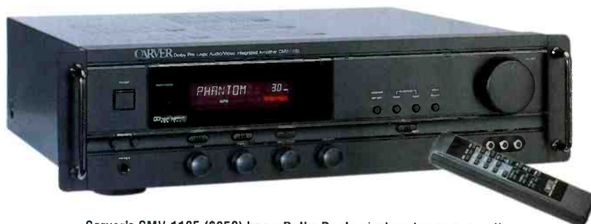
Carver's CMV-1185 ($850) has a Dolby Pro Logic decoder, seven audio inputs, and three video inputs. Rated power output is 80 watts each for the front left and right speakers, 90 watts for the center, and 35 watts each for two surrounds.
