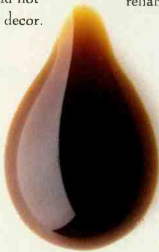
By using a rare ULV Magnetic Fluid to cool a tweeter's voice coil, both performance and reliability are vastly increased.
