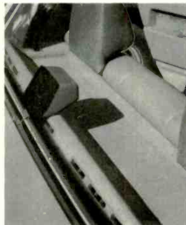
Careful, professional installation, using the original liner material, conceals the subwoofers installed in the rear shelf.
