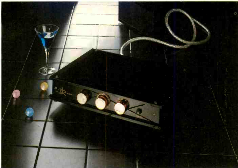
S chäfer and Rompf's ASR Collector preamplifier (left) is housed in a nonmagnetic case made of "acrylic-glass" with solid brass controls.
