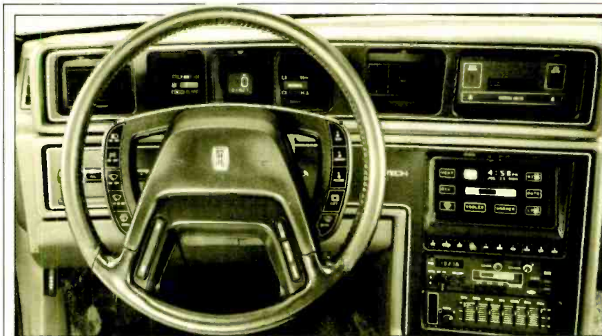
Ford's experimental Mark VII Comtech has audio controls inside the steering wheel.
