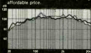
Ambient response and SPL rating for typical Pyle Driver car stereo sound systems
