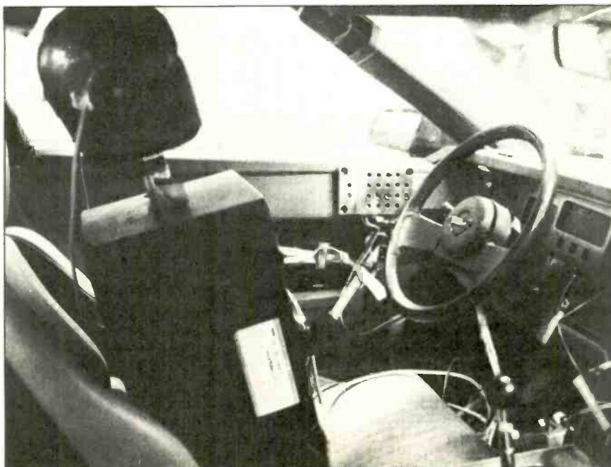
These photos show additional stages in the development of the Delco/Bose car stereo system in the 1984 Corvette. Photo above shows a shell-like mock-up of the car body; note the wood-plank dashboard and roughed-in speaker in the door. The shell's dimensions were close to those planned for the final car, so the Bose engineers were able to experiment with various speaker locations. When the best locations were selected, GM engineers designed the actual doors and rear compartment to accommodate the Bose speaker/amplifier modules. Photo at left shows a later stage, when the structure of the mock-up was closer to the car's final form. Since very small changes in a car's interior can cause major sonic aberrations, the Delco/Bose engineers had to keep readjusting the stereo system until the car reached its final production form.
