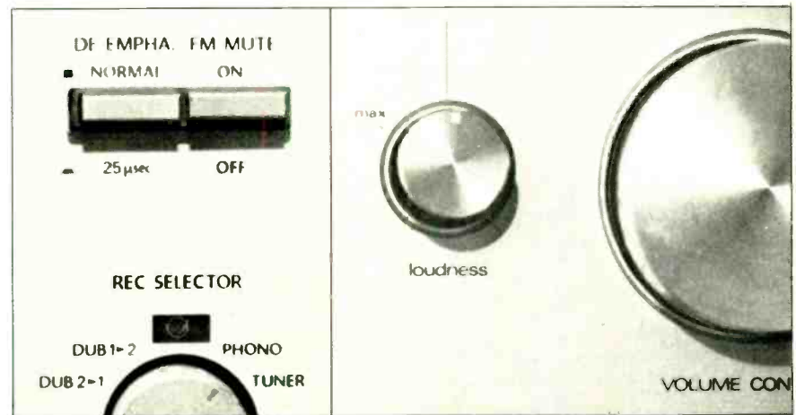
A 25-μsec de-emphasis switch equalizes the signal from Dolbyized FM broadcasts for decoding by an external Dolby processor. A record-selector switch permits listening to one source while recording from another. A loudness control provides needed bass boost at low levels; some variable controls adjust the listening level together with the loudness contour.
