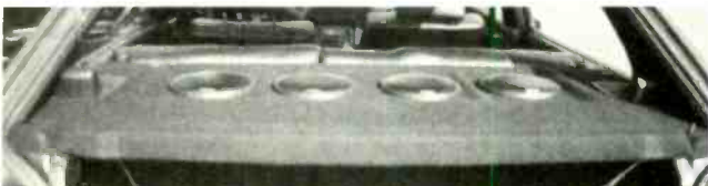
The complete rear system includes four Boston 760LF subwoofers mounted in hinged portion of deck. The 760LFs fit perfectly within the available flat surface on the deck.
