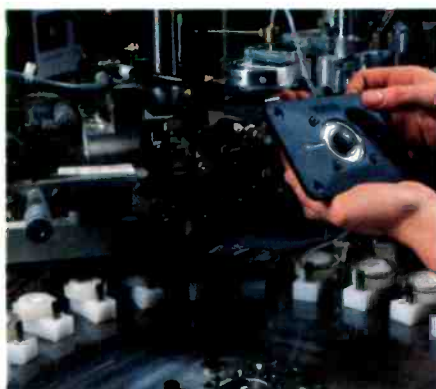
Tweeter voice coils are centered with exacting precision by a sophisticated machine designed and built by Polk Audio engineers.
