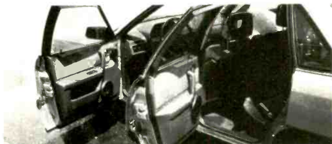
This unusual installation features three-way 763 component systems in front, with 6 1/2" subwoofers installed in doors, Varimount™ tweeters surface-mounted on doors, and 4" midranges in dash. 767 6 1/2" two-way uniaxial systems in rear doors.
