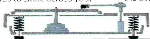
When the base of the PL-630 vibrates, the platter and tone arm don't.
