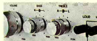
Clutched bass and treble controls with detents.
