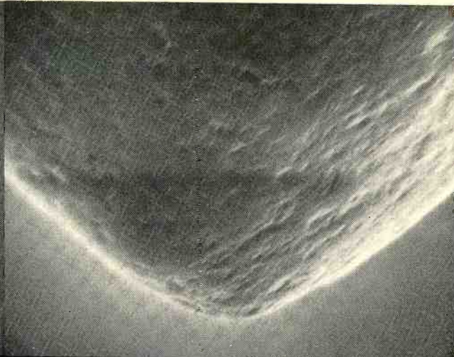
Fig. 6. Under 2,000X magnification a stylus does not appear smooth. "Craters" caused by the diamond dust used as polish are too small to affect performance and disappear after use.
