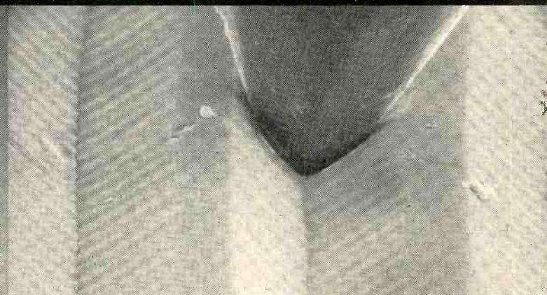
Fig. 2. The latest evolutionary form of stylus is shown tracing the fine groove walls of a CD-4 record. Sharper curvature at contact regions can be seen clearly. Magnification: 2,000X.
