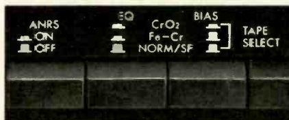
Automatic Noise Reduction System reduces tape hiss.
