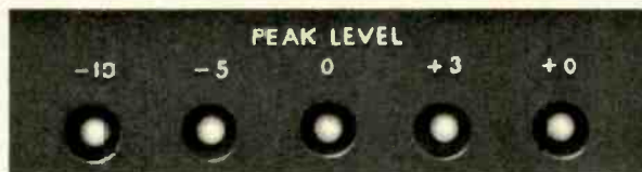
5 LED peak level indicators help eliminate distortion.
