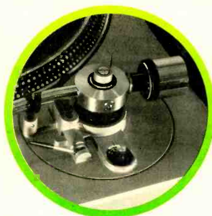
All controls and adjustments for this tone arm are concentrated in the pivot area; this is common for separate arms.
