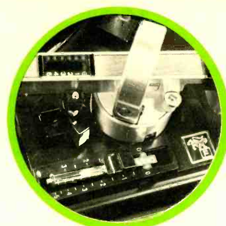
All the new players have separate anti-skating calibrations for conical and elliptical styli, a few for CD-4 types.
