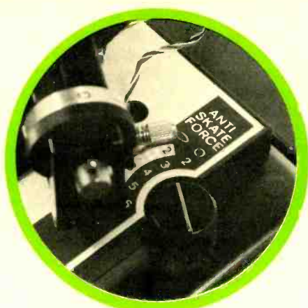
The anti-skating force control can be a rotary knob, an adjustable slider (see right), or a hanging counterweight.
