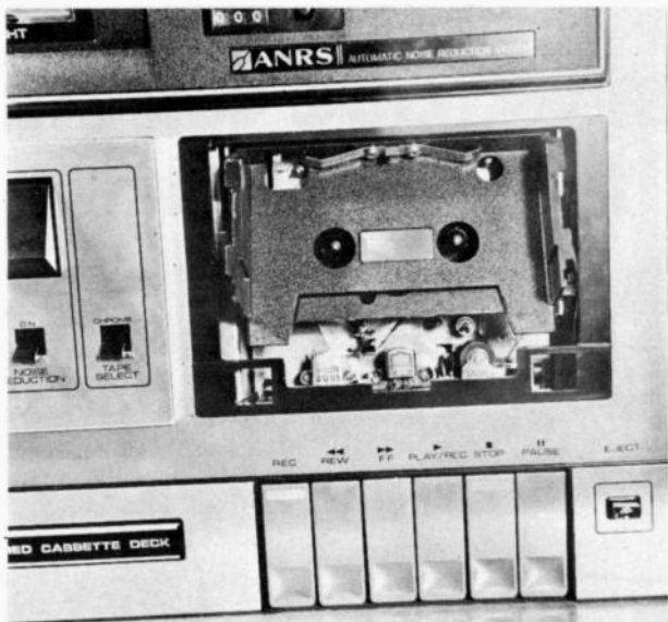
The cover for the 1667's cassette well is completely removable; lifting off another cover plate exposes the heads, capstan, and pinch roller so that they can be easily cleaned and demagnetized.
