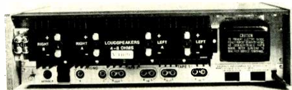
The Tandberg TR-1020 has sockets for DIN speaker connectors in parallel with the speaker-output screw terminals. The inputs and outputs for two tape recorders are below the heat sinks.
