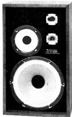
The Kenwood KL-5060 employs four drivers—a cone woofer, cone mid-range, and two tweeters loaded by circular horns—in a three-way configuration.
